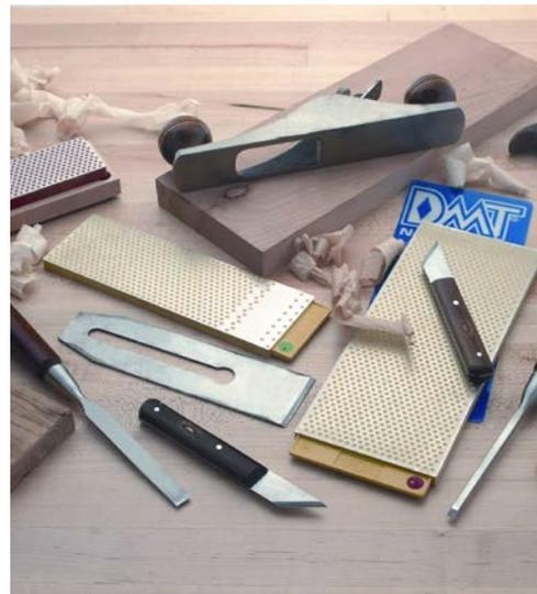
Our DMT Diamond Whetstones save your cash. Your valuable cutter heads last 5–7 times longer than with conventional grinding. The stone consists of many tiny Diamond crystals that are bonded onto a multiholed steel plate. Extreme long life, consistent precise flat surface. Absence of hollows, grooves or depressions and no danger of breakage are distinct advantages. For lubrication a few drops of water are enough – ideal for clean working even on the road.
